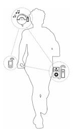
Bluetooth wireless technology is a short-range wireless communication technology intended to replace the cables connecting electronic devices while maintaining the high level of security. With Bluetooth wireless technology, two devices can communicate at the same time without the need to face each other or the concern of interference from other wireless communication within its optimum range of 33 feet.
